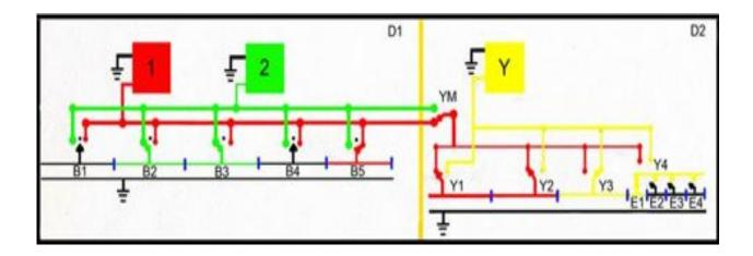
For conventional DC wiring, five electrical blocks that can be controlled independently. Provide one mainline passing siding, one reversing loop, wye, turntable, or transfer table. Have a yard with a minimum of three tracks and a switching lead independent of the main line with facilities for the storing of at least two unused motive power units.
